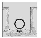
When the conduit(s) are positioned correctly, the trench shall be refilled with sand with a maximum particle size of 20mm and carefully condensed. The area directly on top of the conduit shall be condensed manually up to a height of 0,30 m above the top of the conduit.
