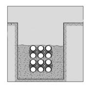
In case the top layer of conduits is less than 0,50 m below the final street surface, additional measurements have to be taken to distribute the traffic load like putting the conduits in concrete or to refill the trench with a mixture of concrete and sand. When putting the conduits in concrete watertight joints have to be used.
