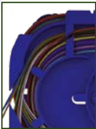
Internal Fibre Management Channels and cross over radius protection
