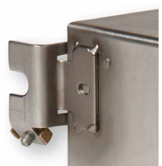
The fastening lugs can be attached in a horizontal or vertical position, or be replaced with threaded inserts. Standard grounding is placed onto one lug.
