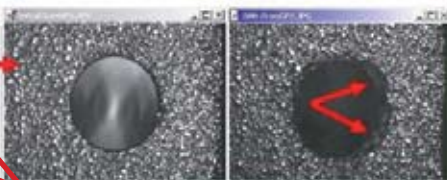
Sharp edged pins cause damage, reducing durability
