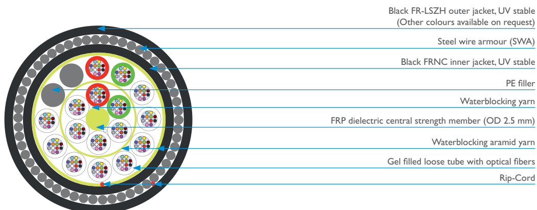
The picture represents a cable with 192 fibers.
