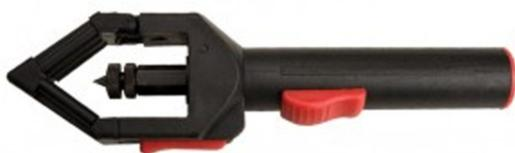
Designed for precision stripping of a variety of insulation types including rubber, PVC, nylon, cotton and coaxial cables from 8mm to 25mm diameter. Its stripping action is both circumferential and longitudinal for the removal of insulation or mid-span wires.
