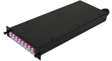
This robust case houses LGX modules for use in LGX 3U chassis. The case allows for up to 24 splices from pigtails to incoming fiber from a cable, it also includes a hole for a cable entry and cable gland. Pre-punched strain tie locations come as standard. The interchangeable LGX modules provide a flexible solution to the user allowing a range of different adapter types.
