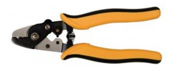
This hard wearing, easy to handle fiber optic stripping tool includes three stripping guides for: 2mm outer jacket, 900µm Buffer, and 250µm acrylic coating, Safety catch and factory set adjuster.
