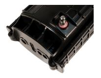
The inline enclosure is suitable for protecting fiber cable splices in straight through and branching applications. Its well-engineered, injection molded outer body makes it impenetrable to the elements. It can protect splices and ensure reliability with usage in ambient temperatures from -40 $^{\circ}$ C to +65 $^{\circ}$ C. It can be placed in aerial, underground, or duct mounted locations.
