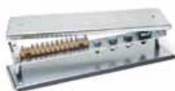
**large version, with terminal bar 35x4 mm, hot-dip galvanised, base plate and cover made of sheet steel. With terminals for: 1 round wire 8–10 mm, 2 flat strip 40x4 mm, 1 copper cable of up to 50 mm<sup>2</sup>, 12 conductors up to 16 mm<sup>2</sup>**
